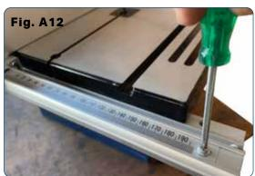
13. Check the table is set at 90° (square) to the blade, using a quality square. If necessary adjust the tilt on the trunnion and lock in place.
