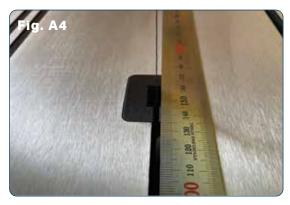
5. Once you are happy with the alignment, go ahead and tighten all the table bolts with the spanner provided. You can then adjust the tilt of the table back to 0°.
